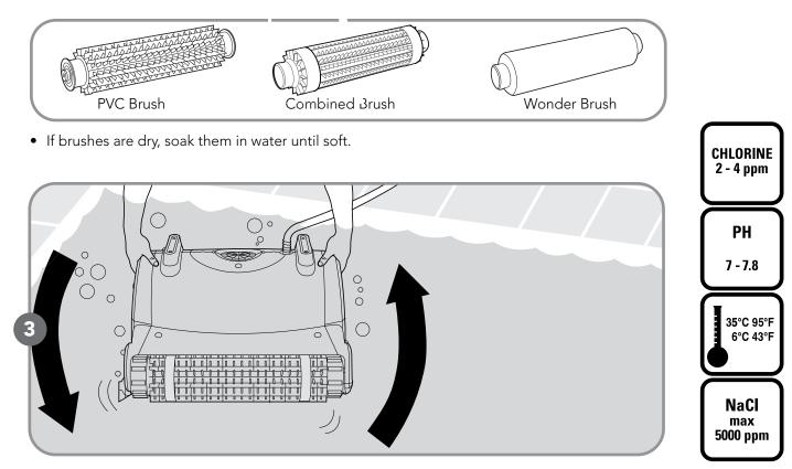
• Shake the robot from side to side or turn it upside down to release trapped air.
